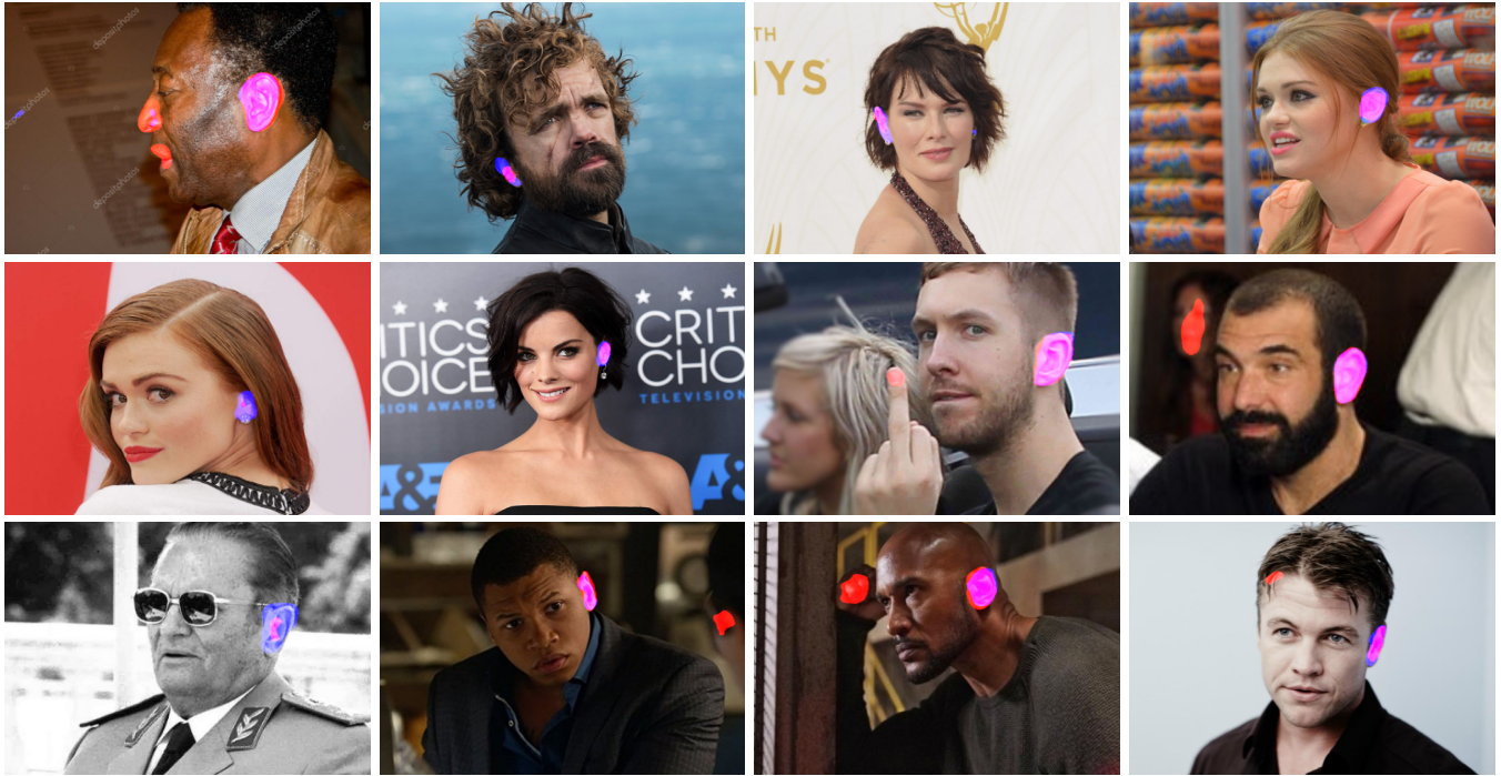
FIGURE 8: Comparison of the segmentation path of ContexedNet trained with and without contextual information. Results are presented with the ResNet backbone model used for implementation of DeepLabV3. Predictions marked red correspond to results without contextual information, predictions in blue correspond to results produced with contextual information, and pink areas correspond to overlapping regions. The figure is best viewed in color.
