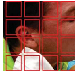
Fig. 1. Red squares represent anchors, which are scanned by region proposal network. These squares are drawn on the original image for illustration. RPN actually scans over the feature maps but areas on the feature maps correspond to areas on original image. These anchors are of different sizes and usually they overlap to cover as much space as possible.
